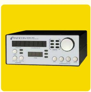
The TF-SQM160 uses proven INFICON guartz crystal sensor technology to measure rate and thickness in thin film deposition processes. Two sensor inputs are standard and four additional sensor inputs are optional. Two recorder outputs provide analogue rate and thickness signals.
