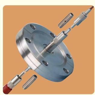
Our fibre optic vacuum feedthroughs are constructed with 100, 200, 400, 600 and 1000  $\mu m$  VIS/NIS fibres, they are designed for vacuum applications requiring fibre optic connection from inside a vacuum system to external equipment. The fibre is hermetically sealed into a stainless steel shell using the latest in glass bonding technology and terminates on both vacuum and air side with standard SMA 905 terminations.
