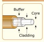
Polyimide buffer fiber is ideally suited for UHV environments and made with step index high-OH silica core for UV/VIS and low-OH silica core for VIS/NIR, doped silica cladding, and a polyimide buffer with a concentricity of  $\pm 3\mu m$ . Fibre is step-index and has a numerical aperture of  $0.22 \pm 0.02$  and a full acceptance cone angle of  $24.8^{\circ}$ . This fiber is supplied non-terminated. Each fiber end is cleaved and NOT polished. Optical fiber has been proof tested to 100 kpsi.
