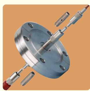
Our fibre optic vacuum feedthroughs are constructed with 100, 200, 400, 600 and 1000 µm UV/VIS fibres, they are designed for vacuum applications requiring fibre optic connection from inside a vacuum system to external equipment. The fibre is hermetically sealed into a stainless steel shell using the latest in glass bonding technology and terminates on both vacuum and air side with standard SMA 905 terminations.
