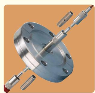
Our graded index fibre optic feedthroughs are constructed with 62.5/125µm core/clad graded-index multimode fibres, they are designed for vacuum applications requiring fibre optic connection from inside a vacuum system to external equipment. The fibre is hermetically sealed into a stainless steel shell using the latest in glass bonding technology and terminates on both vacuum and air side with standard SMA 905 terminations.
