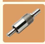
SMA 905 fibre optic connectors are used to terminate UHV and air service fiber optic cables. These connectors mate with corresponding buffer/fibre type as detailed previously. Use of a coupler is required to mate with fibre optic feedthroughs found previously in this catalogue. SMA 905 connectors are made with stainless steel ferrules and bodies for UHV environments.
