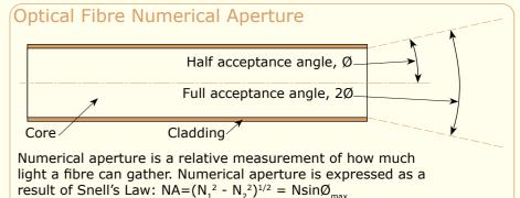
result of Snell's Law:  $NA=(N_1^2 - N_2^2)^{1/2} = Nsin\emptyset_{max}$ . All of our multimode fibres have a numerical aperture of 0.22, which equals a whole acceptance angle of 24.8°
